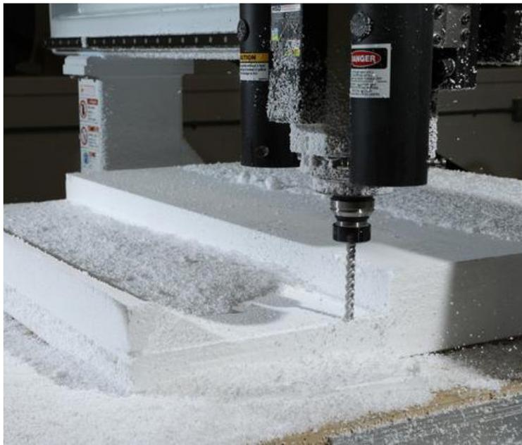
A CNC (computer numeric control) machine cuts modeling foam in the prototype shop. Most of the concepts don't make it to the marketplace. (E. Jason Wambsgans/Chicago Tribune)
